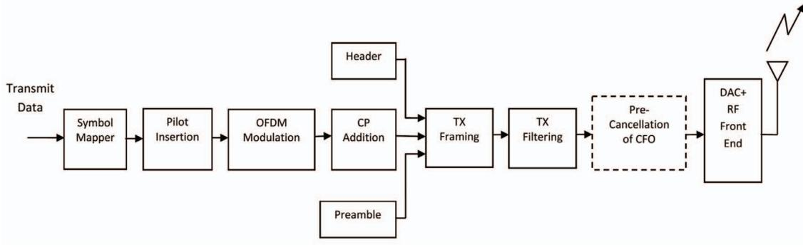
Fig. 1. Block Diagram of Transmitter
