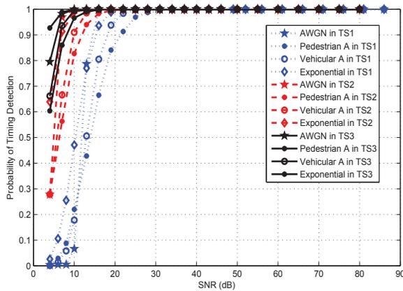
Fig. 5. Performance of Symbol timing algorithm in different time slots: Probability of correct timing detection
