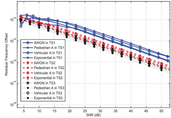
Fig. 6. Normalized Residual Frequency errors in different cooperation phases
