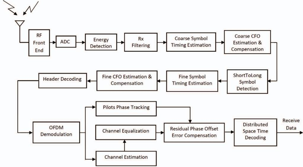
Fig. 2. Block Diagram of Receiver
