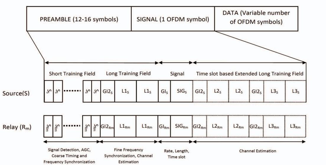
Fig. 3. Transmitter Frame Structure
