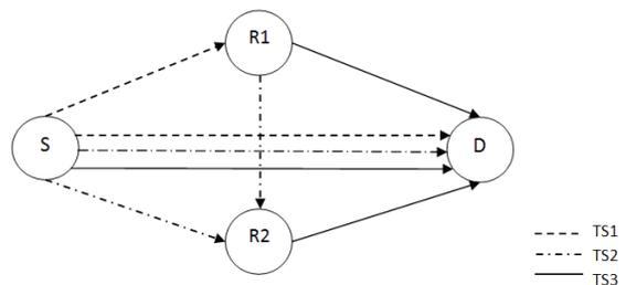
Fig. 4. Schematic representation of Relay assisted Cooperation in different time slots(TS)
